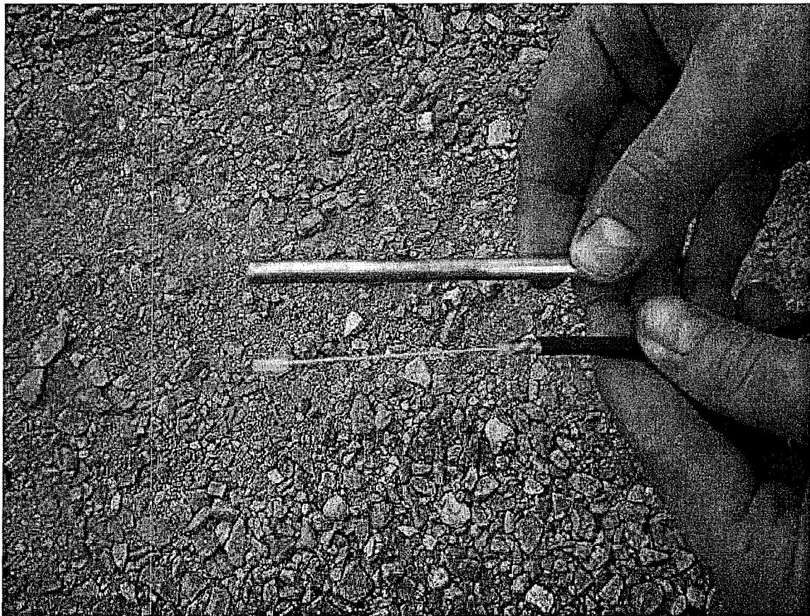
Figure 1: crushable switch (disassembled)
