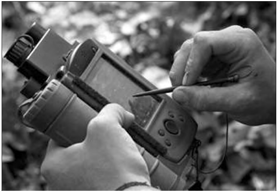
The U.S. Army's XM 32 Lightweight Handheld Mortar Ballistic Computer is a significant improvement over the M23 Mortar Ballistic Computer – its predecessor – because it is lighter, provides digital connectivity to the fire support network, processes ballistic solutions faster, and provides system location through an integrated Global Positioning System.
