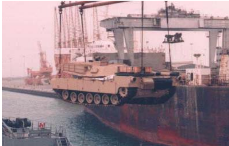
Figure 24: Lifting of M1A1 Main Battle Tank with spreader bars
