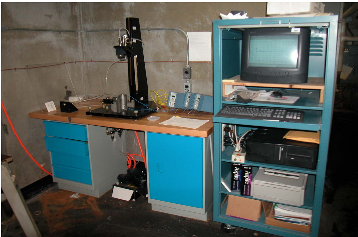
Figure 14c ARDEC Primer Laboratory Sensitivity Test Apparatus
