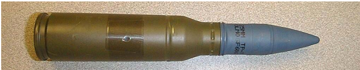
Figure 17. M793 Test Cartridge with Drilled Cartridge Case for Chamber Pressure Measurement
