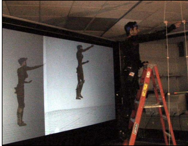
Figure B10: Inertial Suit Vertical Translation Error
