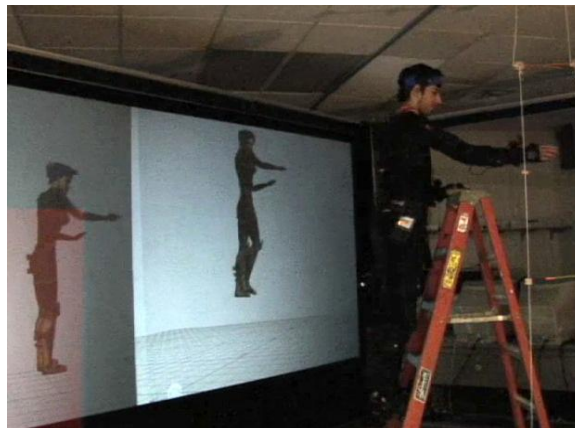
Figure B2: Climbing a Ladder Test The left avatar is the 3DSuit, right is the ReActor2
