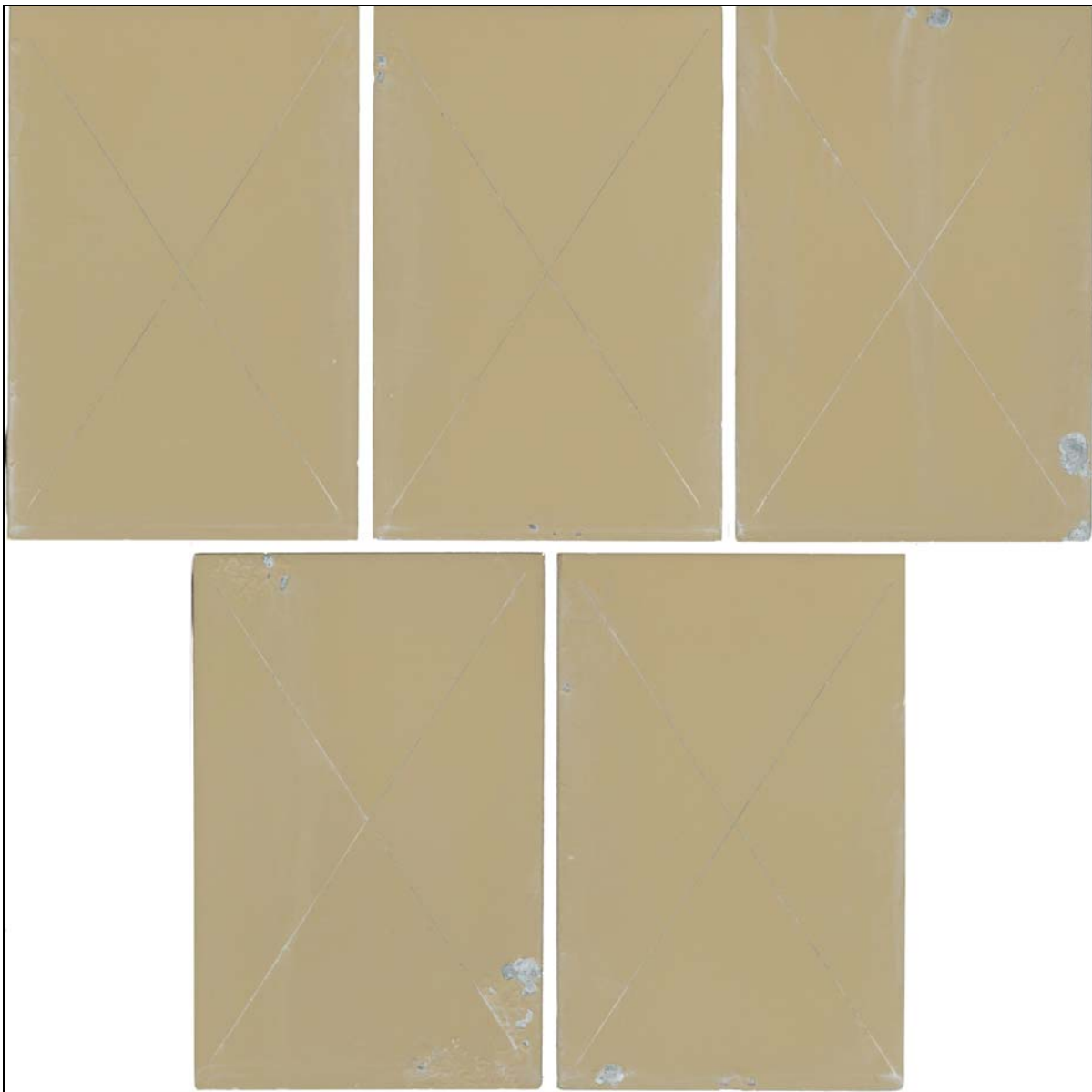
Figure 8. All five replicates prepared by abrasive blast after 8760 hr (1 year) NSF exposure, blisters along scribe and attack at panel edges.
