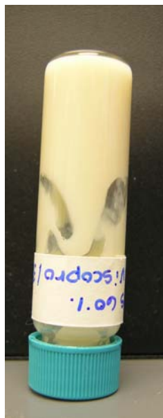
Figure 21. 8% Viscoprop S.F. and 32% Tap Water in Gas Without Ethanol
