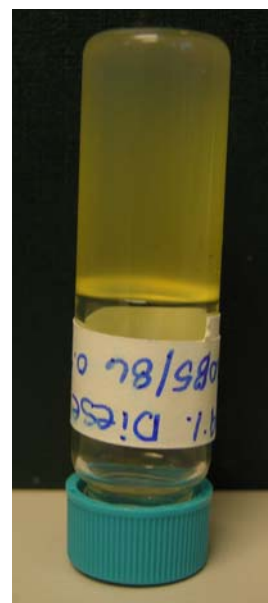
Figure 13. 0.5% Each MO-85M and MO-86M in Diesel Fuel
