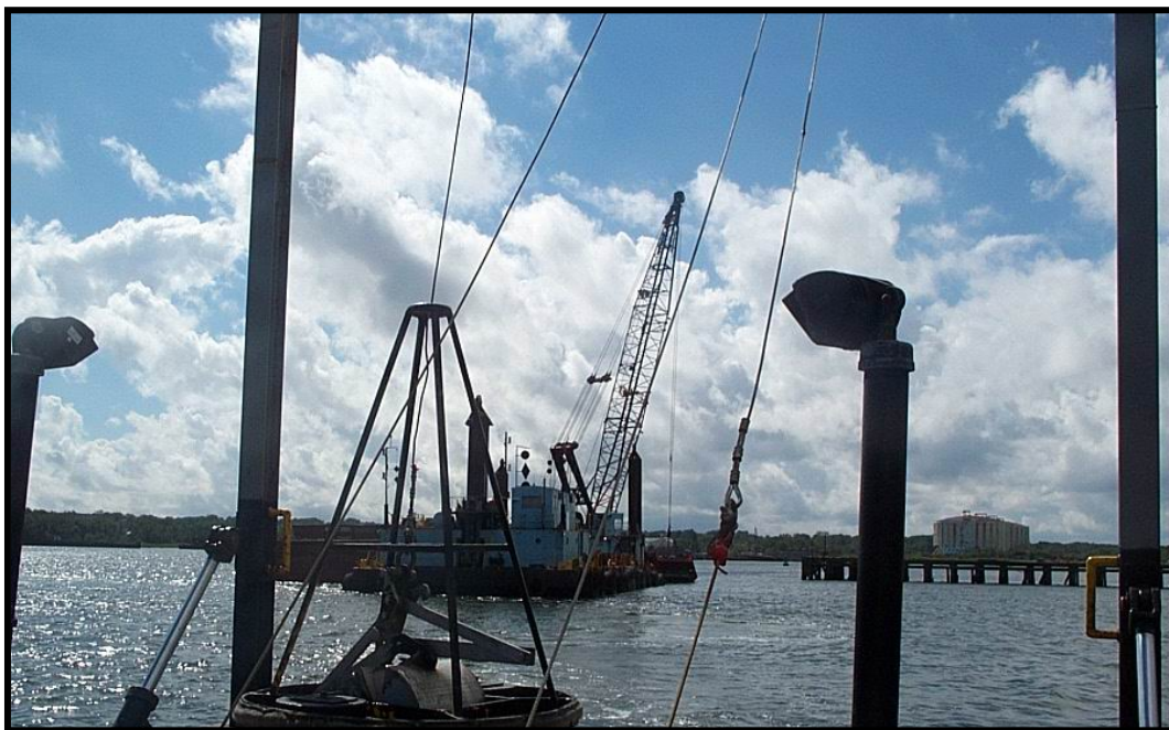
Figure 2. Van Veen grab used in collection of the sediments. Picture was taken at the Arthur Kill sampling location.
