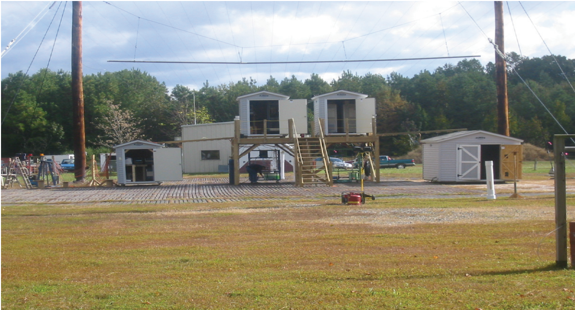
Figure 1-4. EMP Simulator with Test Structures and Internal Electronics
