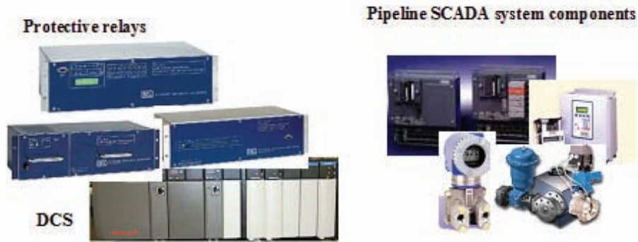
Figure 1-5. Some of the Electronic Control Systems Exposed in Test Facility
