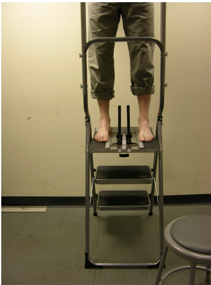
Figure 2. Device Used to Measure Foot Arch Height
