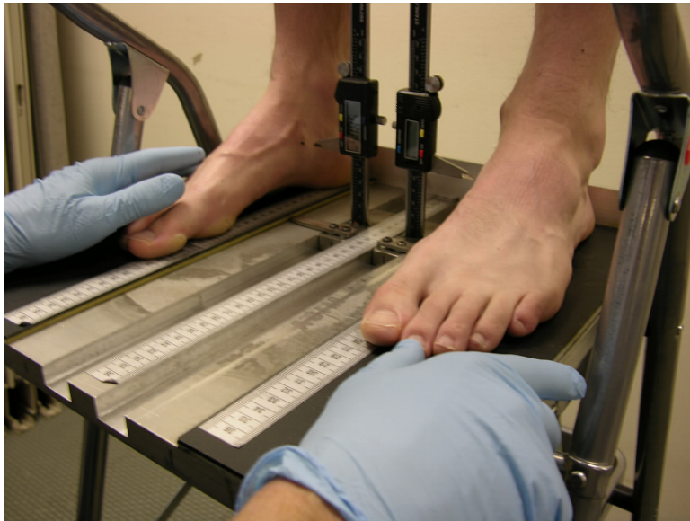
Figure 3. Foot Length and Arch Height Measurements Being Taken on a Subject
