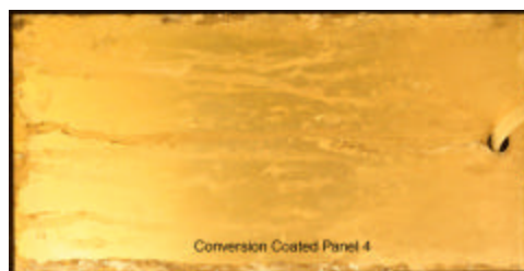
Figure 74: Unscribed conversion-coated Al panel after 616 hours of exposure.
