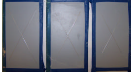
Figure 128: Al 2219-T87 with BAM-PPV + Mil-PRF-23377 + Mil-PRF-85285 2560 hours of exposure
