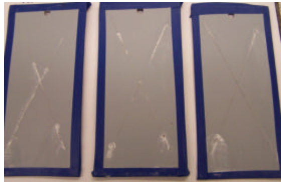
Figure 112: TCP + Mil-P-53022 + Mil-PRF -85285 on Al 2024-T3 2000 hours of exposure
