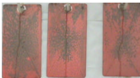
Figure 68: Steel panels after 41 hours of salt spray exposure.
