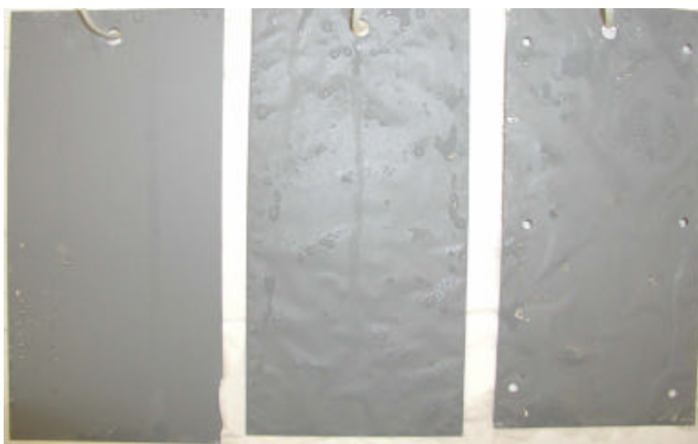
Figure 80: Failure of Al panels coated with flame deposition process after an exposure time of 19 hours.
