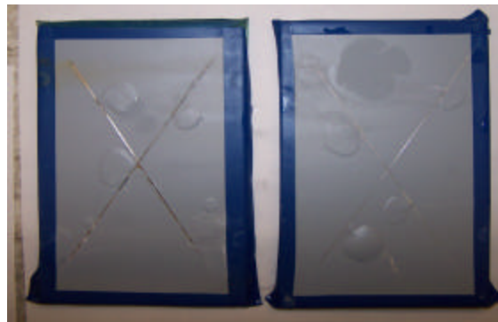
Figure 126: Al 2219-T87 with BAM-PPV +Mil- P-53022 + Mil-PRF-85285 500 hours of exposure
