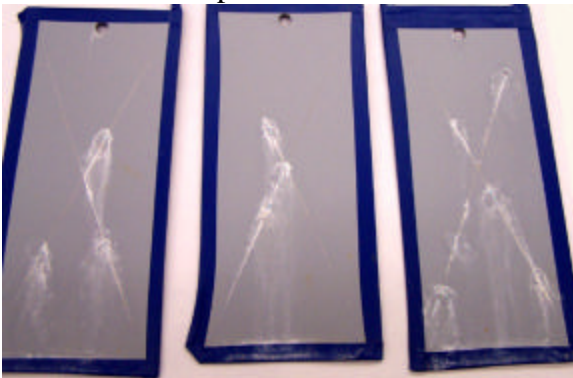
Figure 114: CCC + Mil-P-53022 + Mil-PRF-85285 on Al 2024-T3 2000 hours exposure
