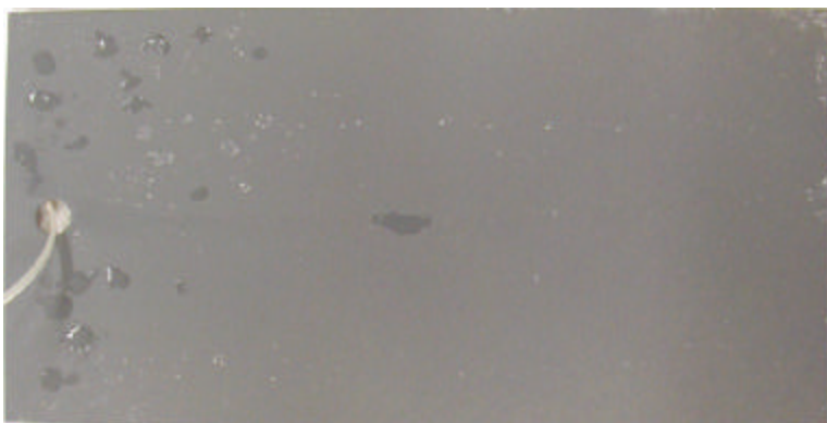
Figure 82: Panel coated with BAM-PPV/primer/topcoat. Visible spots are water droplets on the surface.
