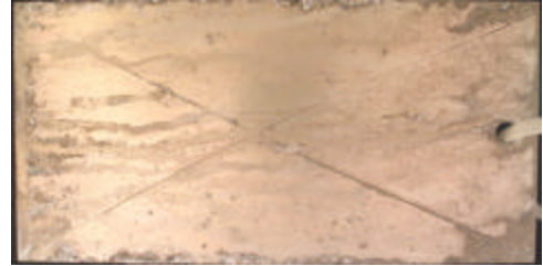
Figure 76: Scribed conversion coated Al panel (1146 hours of exposure).
