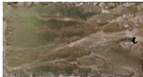
Figure 79: Scribed conversion coated Al Panel (3000 hours of exposure).
