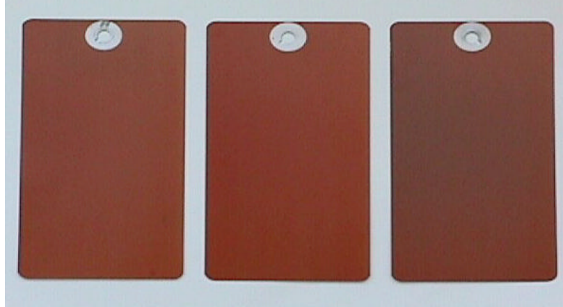
Figure 51: Steel panels (3'x 6') coated with BAM-PPV using the flame deposition process
