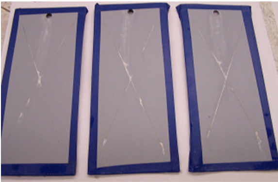
Figure 111: BAM-PPV + Mil-P-53022 + + Mil-PRF-85285 on Al 2024-T3 2000 hours of exposure
