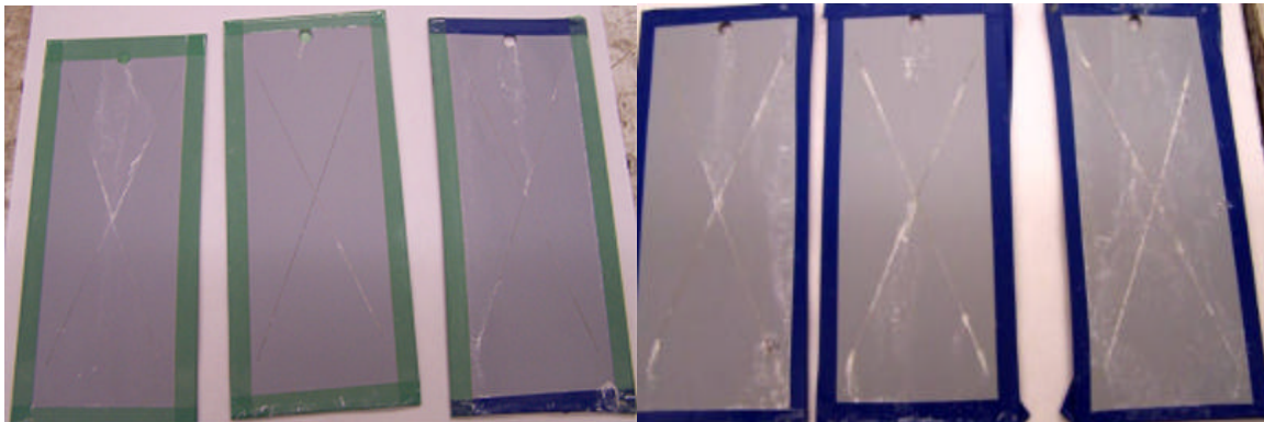
Figure 119: Alodine 5700 + Mil-PRF-85582 (N) + Mil PRF-85285 on Al 2024-T3 2000 hours of exposure
