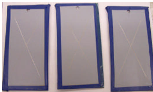
Figure 123: CCC + Mil-PRF-23377 + Mil-PRF-85285 on Al 2024-T3 2000 hours of exposure
