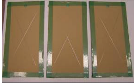
Figure 130: Al 2024-T3 with BAM-PPV + Mil-P-53030 + Mil-C-46168 1250 hours of exposure
