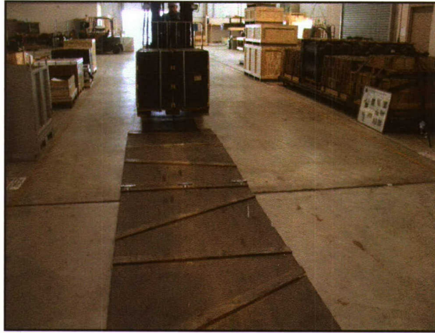
Photo 12. Forklift Testing of the Test Unit.
