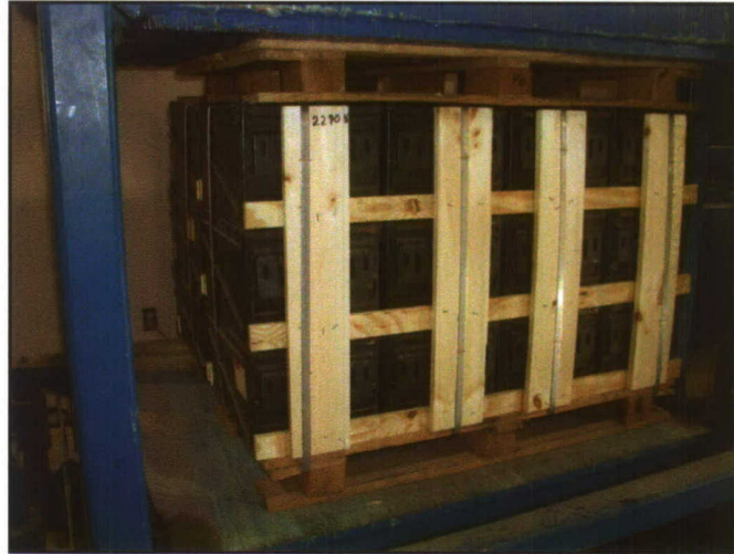
Photo 7. Test Unit in the Stacking Test.
