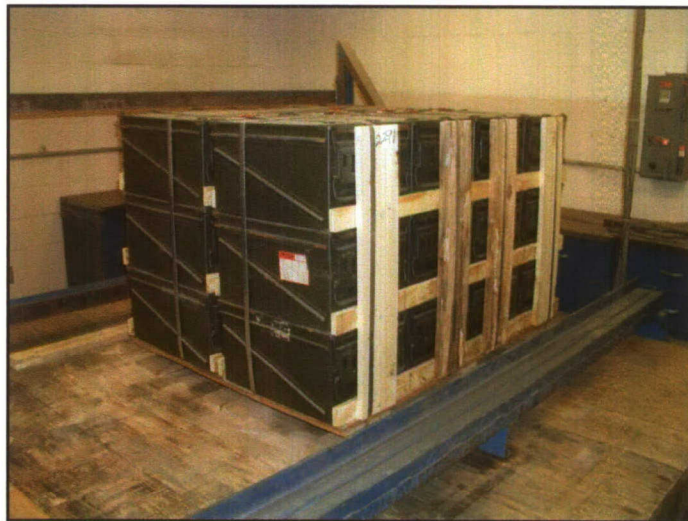
Photo 8. Test Unit During Repetitive Shock Testing.
