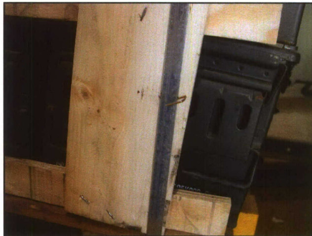
Photo 11. Disengaged Staple During Incline-Impact Testing of Test Unit #1.
