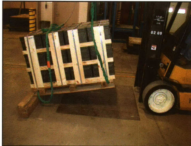
Photo 9. Edgewise Drop Test on the Test Unit.
