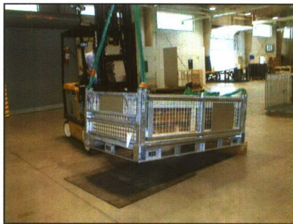
Photo 3. Example of Edgewise-Rotational Drop Test (MSTF Low)
