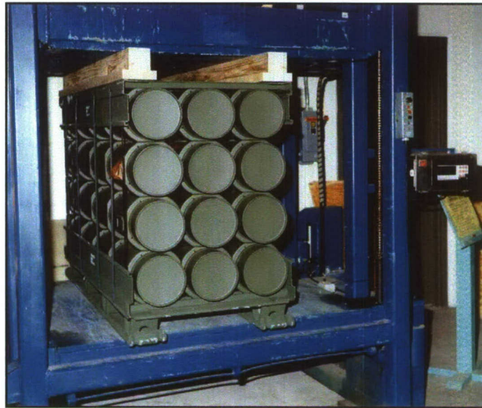
Photo 1. Example of Stacking Test. (2.75-inch Hydra 70, PA151 Rocket Pallet in the Stacking Test.)
