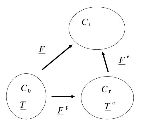
Fig.3: Decomposition of the deformation gradient  $\underline{F}$  into plastic part  $\underline{F}^{\rm p}$  and elastic part  $\underline{F}^{\rm e}$ .
