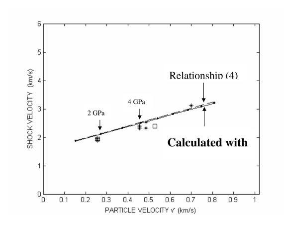
Fig.2: Shock velocity C versus particle velocity  $v^-$  at the rear of the plastic shock. Experimental data are represented by stars and squares respectively for PC37/SS19 and PC74//SS37 laminates. The dashed line is given by equ. (4) with slope S=2.1,  $v^+=18.2m/s$  and  $c^+=1600m/s$ . The solid line with dots corresponds to calculations made in section 4.2 by using the Hugoniot defined by (39)
