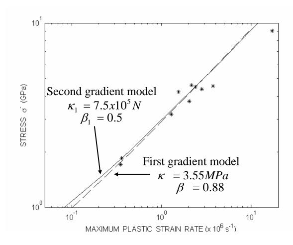
Fig.18: First gradient approach ( $\beta = 0.88$ ,  $\kappa = 3.55$  MPa) compared to second gradient approach ( $\beta_1 = 0.5$ ,  $\kappa_1 = 7.5x10^5$  N), respectively dashed and solid lines. Stars represent experimental data for PC37/SS19.
