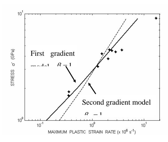
Fig.15: Compared to the first gradient model, the slope of the (dashed) line associated to the second gradient model (with  $\beta_1=1$ ) is not adequate to account for experimental results of PC37/SS19 (stars)
