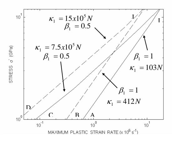
Fig.16: Second gradient approach: effects of parameters  $\beta_1$  and  $\kappa_1$  on the relationship between stress amplitude and magnitude of plastic strain rate. The slope depends on the value of  $\beta_1$  but is not dependent upon  $\kappa_1$ . For a given value of  $\beta_1$ , the lines are shifted horizontally by changing the value of  $\kappa_1$ .
