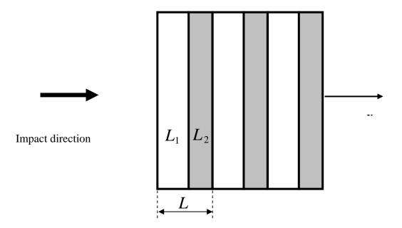
Fig.1: Schematic of the geometry of a periodically layered composite with layer's thicknesses  $\ L_1$  and  $\ L_2$
