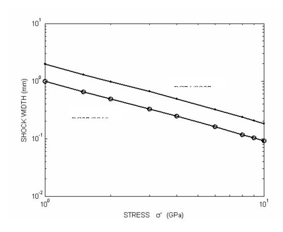
Fig.11: Shock width westimated with (55). Note that the shock width for PC74/SS37 is twice that for PC37/SS19. Dots correspond to the following stress amplitudes (Gpa): 1, 1.5, 2, 3, 4, 6, 8, 9, 10.
