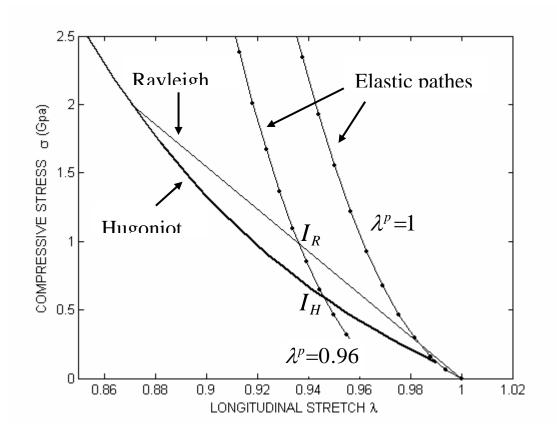
Fig.7: The elastic loading path corresponding to the fixed value of the plastic stretch  $\lambda^p$ =0.96 intercepts the Hugoniot at  $I_H$  and the Rayleigh line at  $I_R$ . The shock stress amplitude is  $\sigma^-$ =2GPa.
