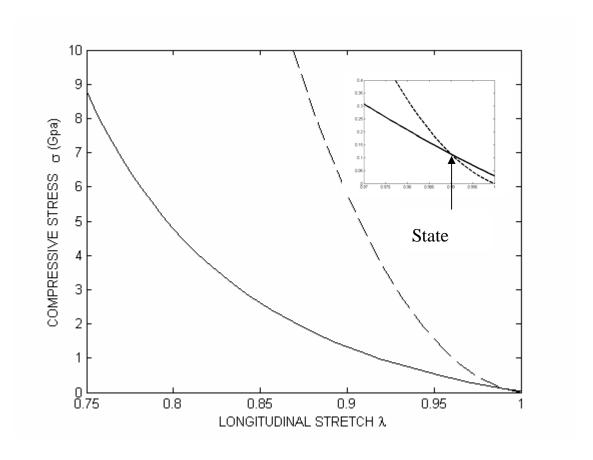
Fig.5: Hugoniot curve (solid line) and elastic loading path  $\lambda \rightarrow \sigma = -T_{11}(\lambda, 1)$  (dashed line) for the laminate PC37/SS19. Results are identical for PC74/SS37. A zoom is shown for  $0.97 \le \lambda \le 1$  in the upper part of the figure.
