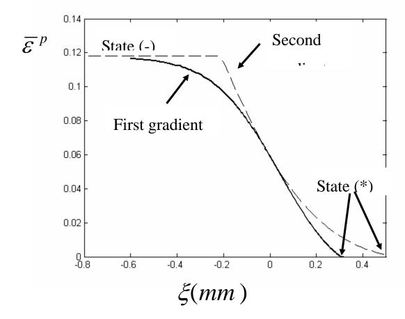
Fig.13: Distribution within the shock structure of the cumulated plastic deformation  $\bar{\varepsilon}^p$  in terms of the position. The first gradient plasticity theory defined by (48) with ( $\beta=1$ ,  $\kappa=1.7m.MPa$ ) is compared to the second gradient theory (60) with ( $\beta_1=1$ ,  $\kappa_1=750N$ ). The stress amplitude is  $\sigma^-=2GPa$ .
