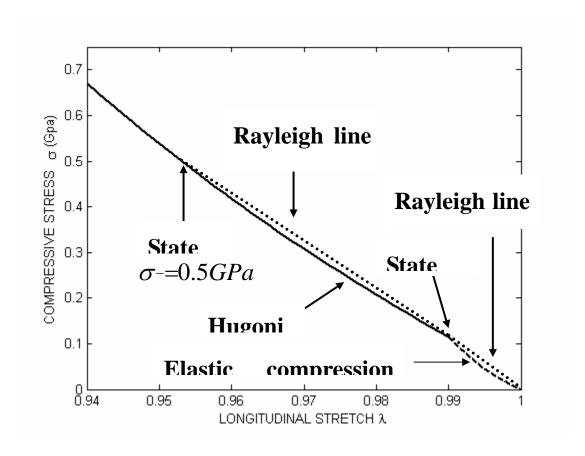
Fig.4: Plastic shock for the stress amplitude  $\sigma$ -=0.5GPa. The material is first compressed from the initial state to the state (+) by an elastic shock (elastic precursor), and is further compressed by a plastic shock from state (+) to state (-). These two distinct shocks exist if the condition (41) on shock velocities is satisfied.
