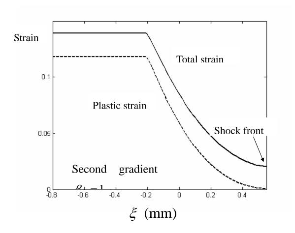
Fig.14: Shock wave profiles calculated for  $\sigma^-=2GPa$  with the second gradient approach  $(\beta_1=1,\kappa_1=750N)$ . The dashed and the solid lines correspond respectively to distributions of the plastic strain  $\overline{\varepsilon}^p$  and of the absolute value of the total strain  $|\varepsilon|=|\log(\lambda)|$ .
