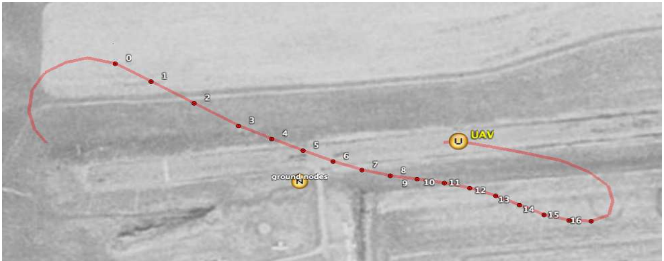
Fig. 1. A U.S. Geological Survey (USGS) satellite map showing the location of an elevated ground node (N), node 3 in Figure 5, and a sample UAV path in a fly test. The horizontal, light-colored band under the UAV node (U) is the airport runway, which is approximately 25 yards wide. The dots show the positions reported by the GPS once a second.
