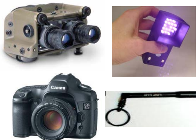
Fig. 2: Interrogation and detection equipment is simple and readily available and includes (a) night vision goggles, (b) near IR cameras, (c) IR flashlights, and (d) flashlights/laser pointers.
