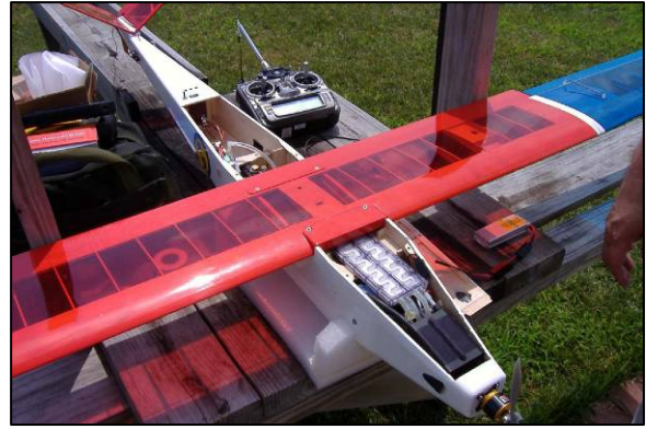
Figures 5: NRL's Spider Lion UAV powered by Protonex fuel cell system
