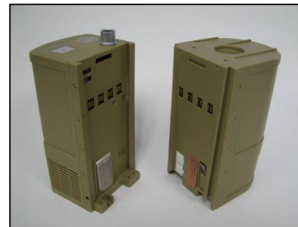
Figure 3: Protonex P2 system showing fuel cell (left) and cartridge (right) components
