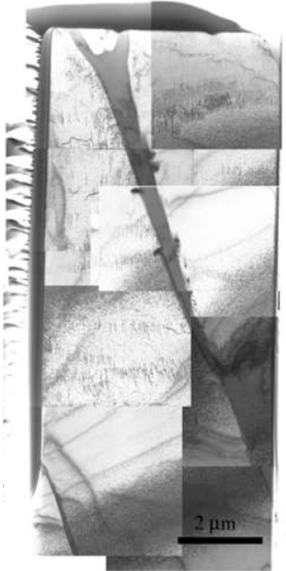
Figure 16. BF-TEM images taken from a 5 μm Ti-6242 longitudinal foil, such that the Burgers vector is out of the plane of the foil.
