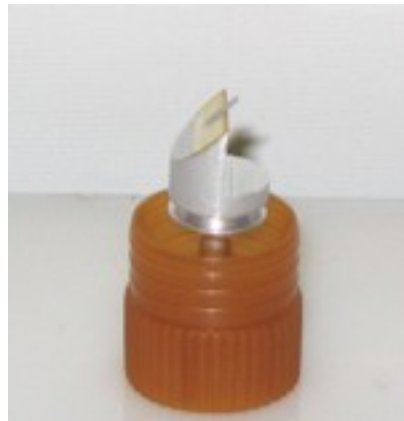
Figure 3: Sample mounted on 45 degree pre-tilted holder.
