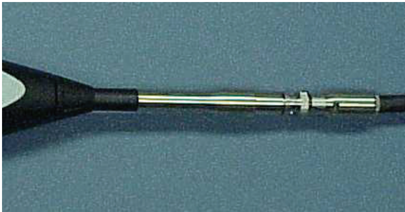
Figure 6. The connection between the USLM system with the two adapters and hydrophone cable is shown.
