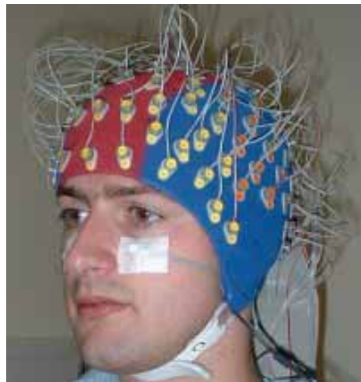
Figure 2.17. BioSemi 128-channel active EEG system (courtesy of BioSemi).
