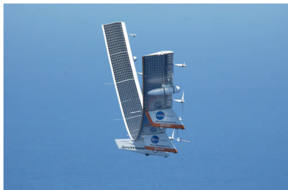
Figure 5: HP03-2 with high wing dihedral
