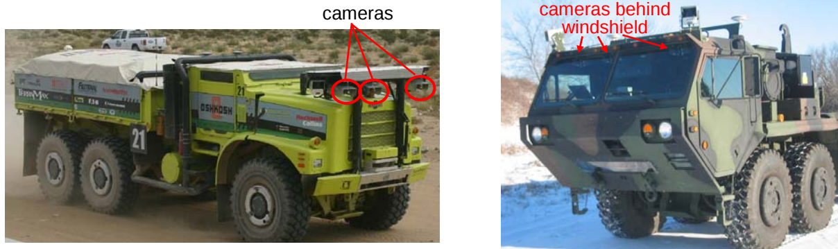
Figure 10: Oshkosh Truck unmanned vehicles: TerraMax™, based on MTRV, (left) and autonomous PLS (right)
