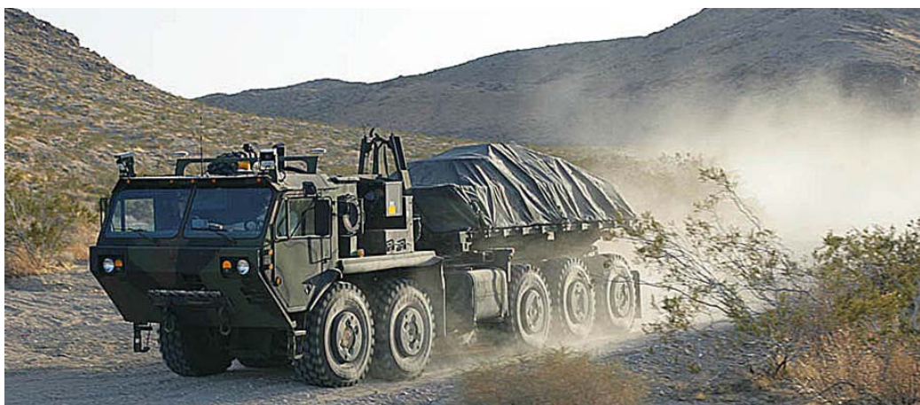
Figure 9: Autonomous PLS operating off-road with full load
