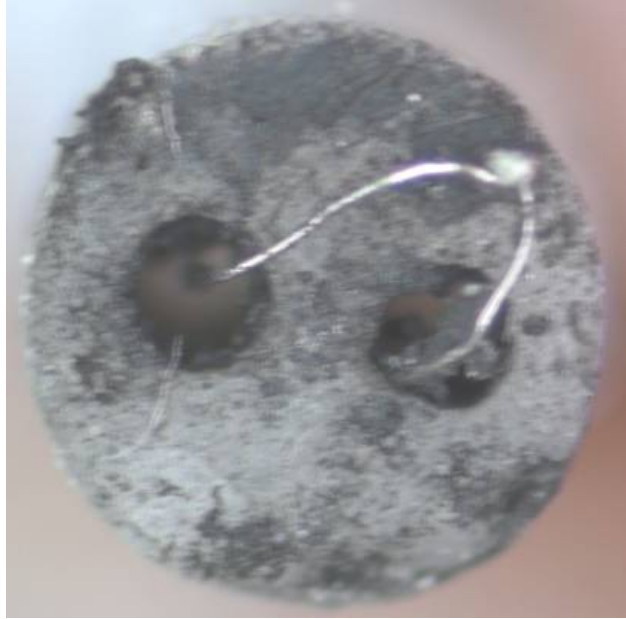
Figure 6. Photograph of 1-mil thermocouple junction mounted with ceramic tube after venting event.
