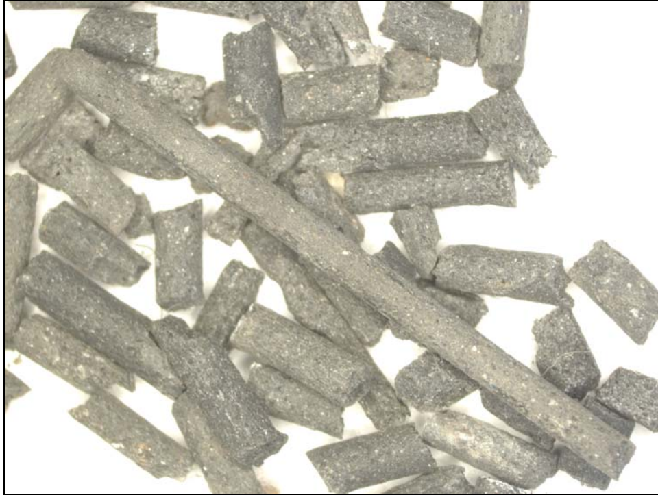
Figure 22. Photograph of pieces of benite found on floor after experiments (origin from M129 or M125 unknown, long piece probably from M129 due to length).
