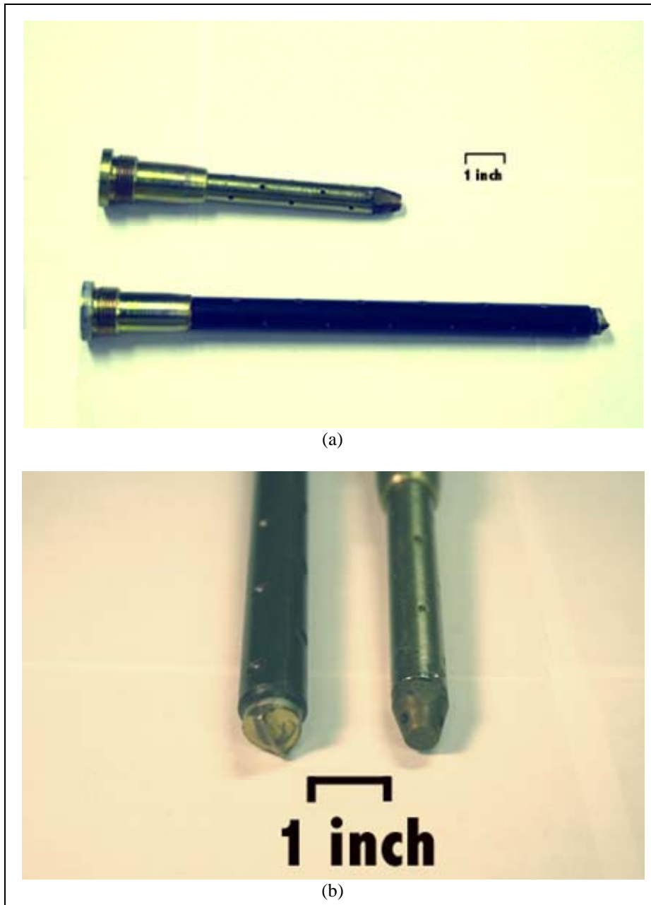
Figure 1. Photographs of (a) M129 (taper tip) and (b) M125 (black rubber coated) primers.
