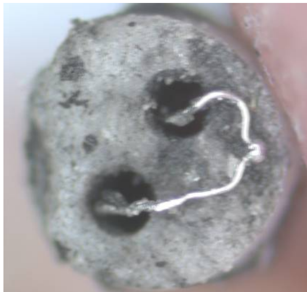
Figure 7. Photograph of 2-mil thermocouple junction mounted with ceramic tube after venting event.
