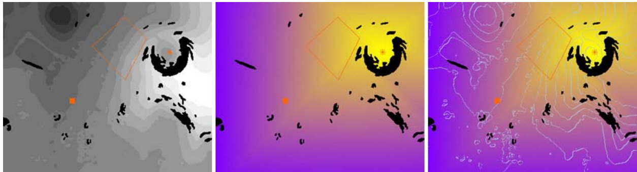
Figure 5.4 Possible map visualizations, including start & goal locations and designated way-area. From left to right, (a) elevation contours visualization, (b) levels of equal cost visualization, and (c) both visualizations.
