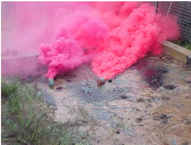
Figure 8. Side-by-Side Comparison of New M18 Red Smoke Mix with Standard M18 Red Grenade.
