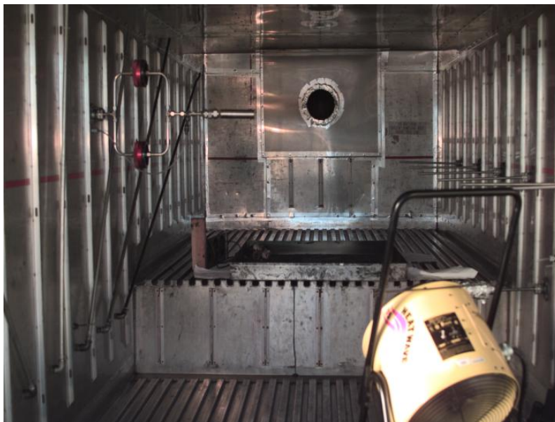
Figure 4. Inside the Smoke Characterization Test Chamber.
