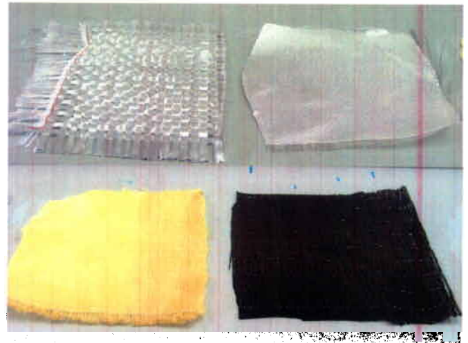
Figure 5: Top: 24oz (left) and 8oz (right) S-2 fiber glass. Bottom: Kevlar (left) and Graphite (right)
