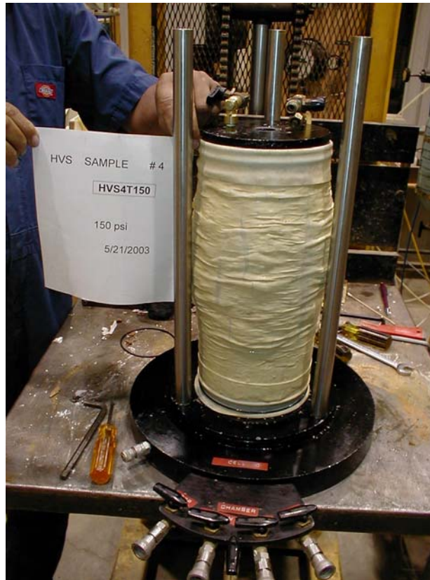
Figure 11. View of final membrane around specimen seen after failure.
