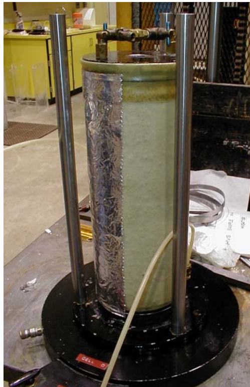
Figure 9. Application of thicker outer latex membrane and aluminum foil strips to specimen to reduce air diffusion.
