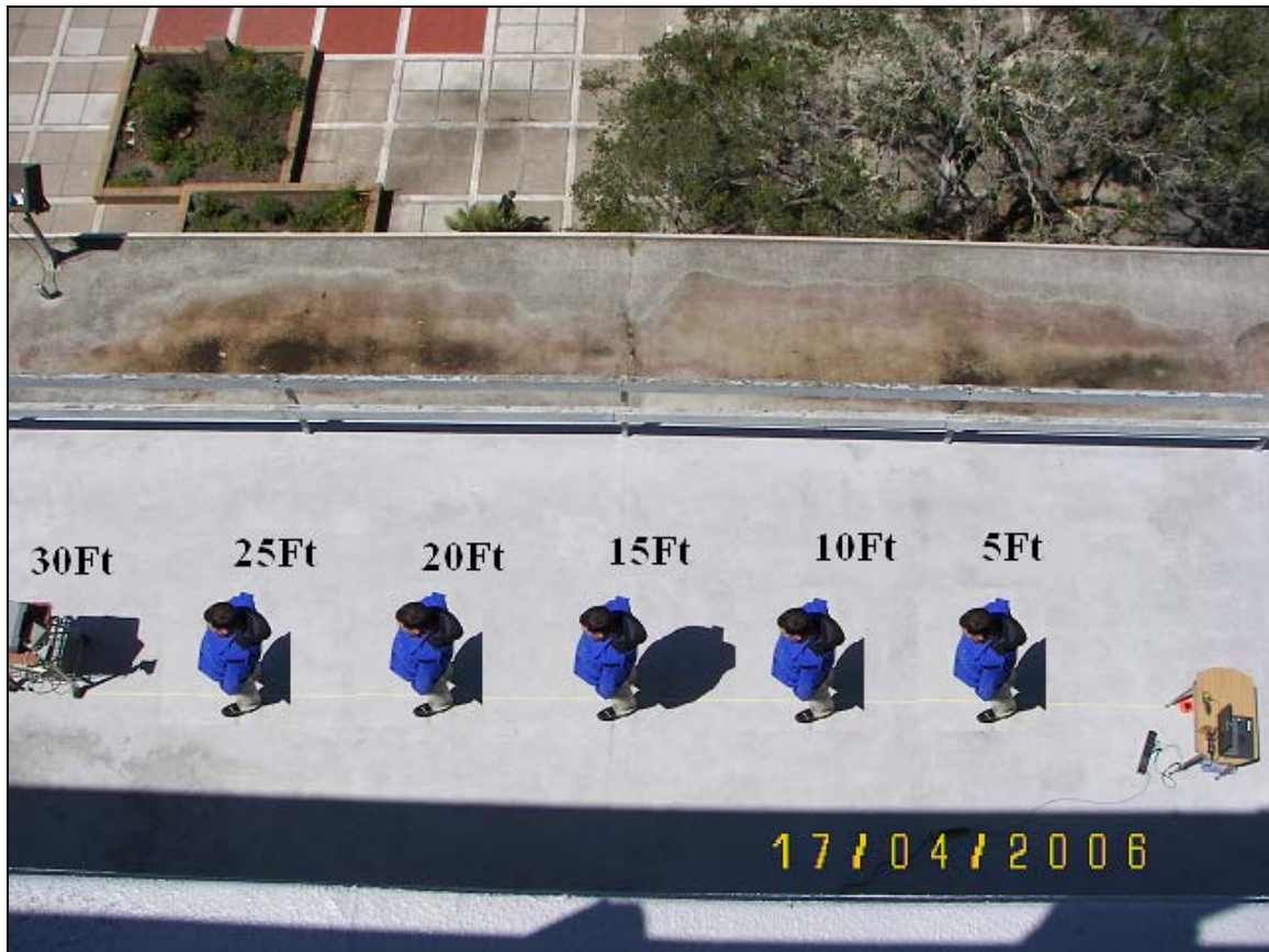
Figure 28. The Experimental Setup for Human Presence between Transmitter and Receiver.
