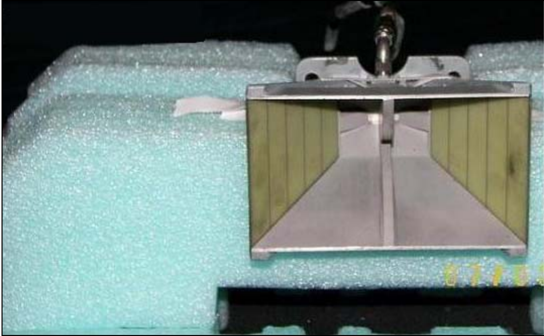
Figure 23. The AEL Pyramidal Horn Antenna at the Anechoic Chamber Gain Measurement.
