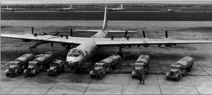
The controversial B-36 carried over 21,000 gallons of gasoline and 1,200 gallons of oil when fully loaded. ( NASM photo )
