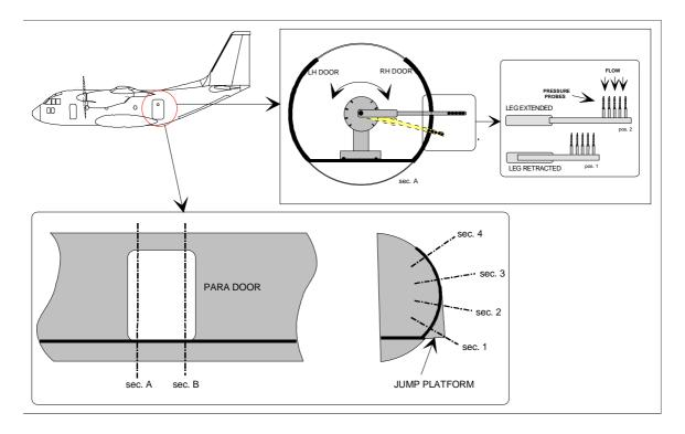
In the earlier phase an "aerodynamic field measurement system" was flown, designed and manufactured in house, to map the airflow characteristics just outside the doors where the paratroops is firstly invested during jump.
