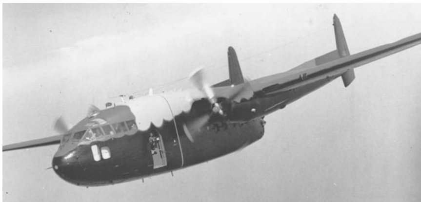
Gunships. Gunship I, an AC-47 (top ), carried three 7.62-mm miniguns; the Gunship II prototype, an AC-130A (center), had four 7.62-mm miniguns and four 20-mm guns; the AC-119G, Gunship III, (bottom), had four 7.62-mm miniguns.
