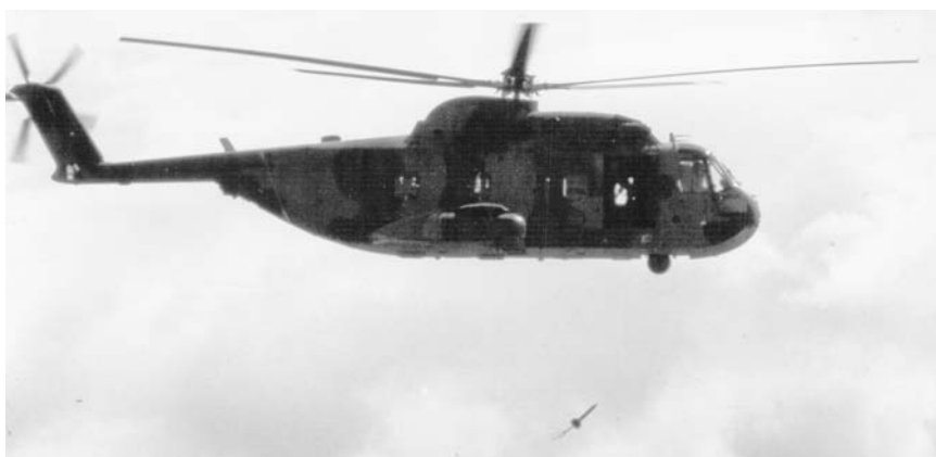
Sensors. A seismic sensor is attached to a pylon on a Navy OP-2E (top), an OP-2E releases a sensor (center), and a CH-3 releases a seismic sensor (bottom).
