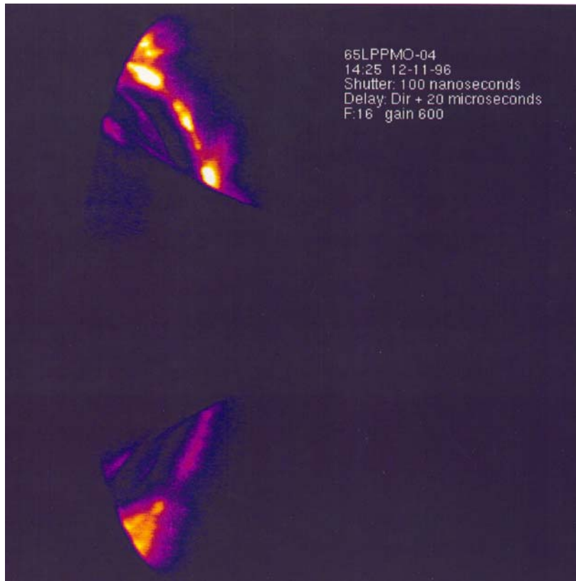
Fig. 36. Example of High Speed Photography Showing Plasma Breakdown on the Inside of the Shroud (Outline of Parabolic Reflector can be Seen in Center of Picture)
