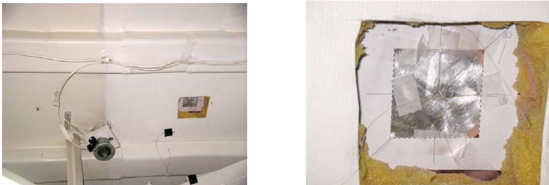
Figure 2: One of the FBG rosettes installed on the deckplate below the foam insulation. Insulation was removed with a knife, the deckplate was sanded down to create a bare aluminum surface. Each FBG rosettes consists of 3 gratings measuring strains at 0, 45, and 90 degrees relative to the longitudinal axis of the ship ( 0^{\circ} ).
