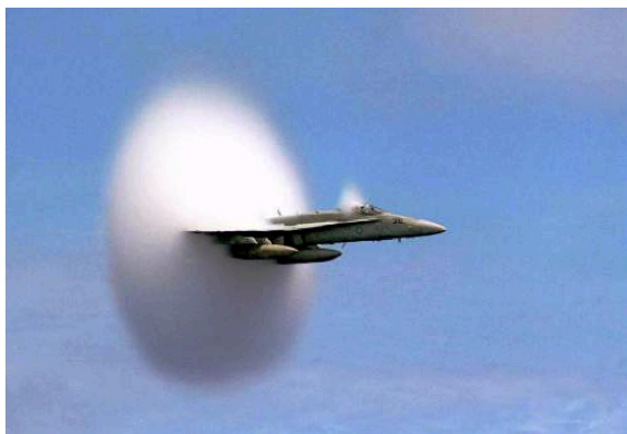
Figure 12.4: F-18 shock waves: Shock waves behind the canopy and along the wings and fuselage of an F-18 fighter jet the instant it breaks the sound barrier.
