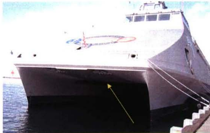
Figure 19. Schematic showing the bottom of the hull that required impact to define a slam event.
