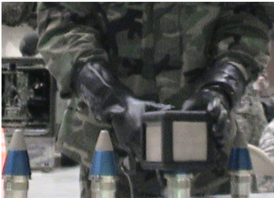
Figure 9. Participant, while wearing modified MOPP IV equipment, setting the second MOFA fuze after setting the first MOFA fuze on the left.
