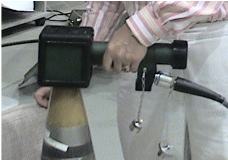
Figure 8. EPIAFS setter being held on excalibur fuze for setting.
