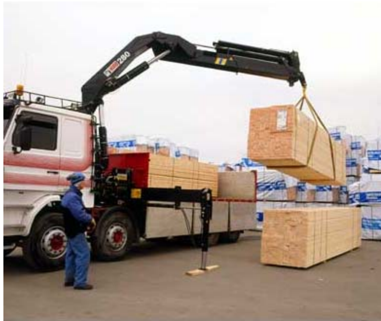
Figure 18: Hiab 280 Truck Mounted Crane
