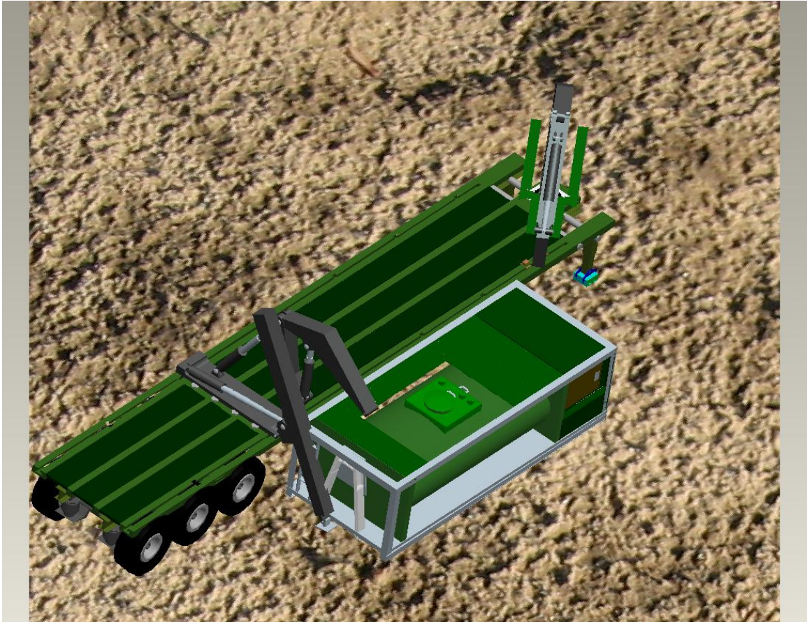
MFT Cranes in Position to Lift Water Tank Flatrack
