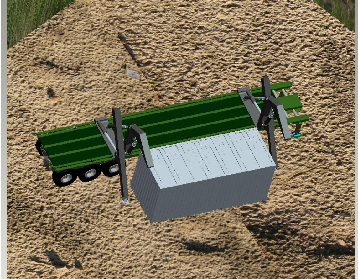
MFT Cranes in Position to Lift 20 foot ISO Container
