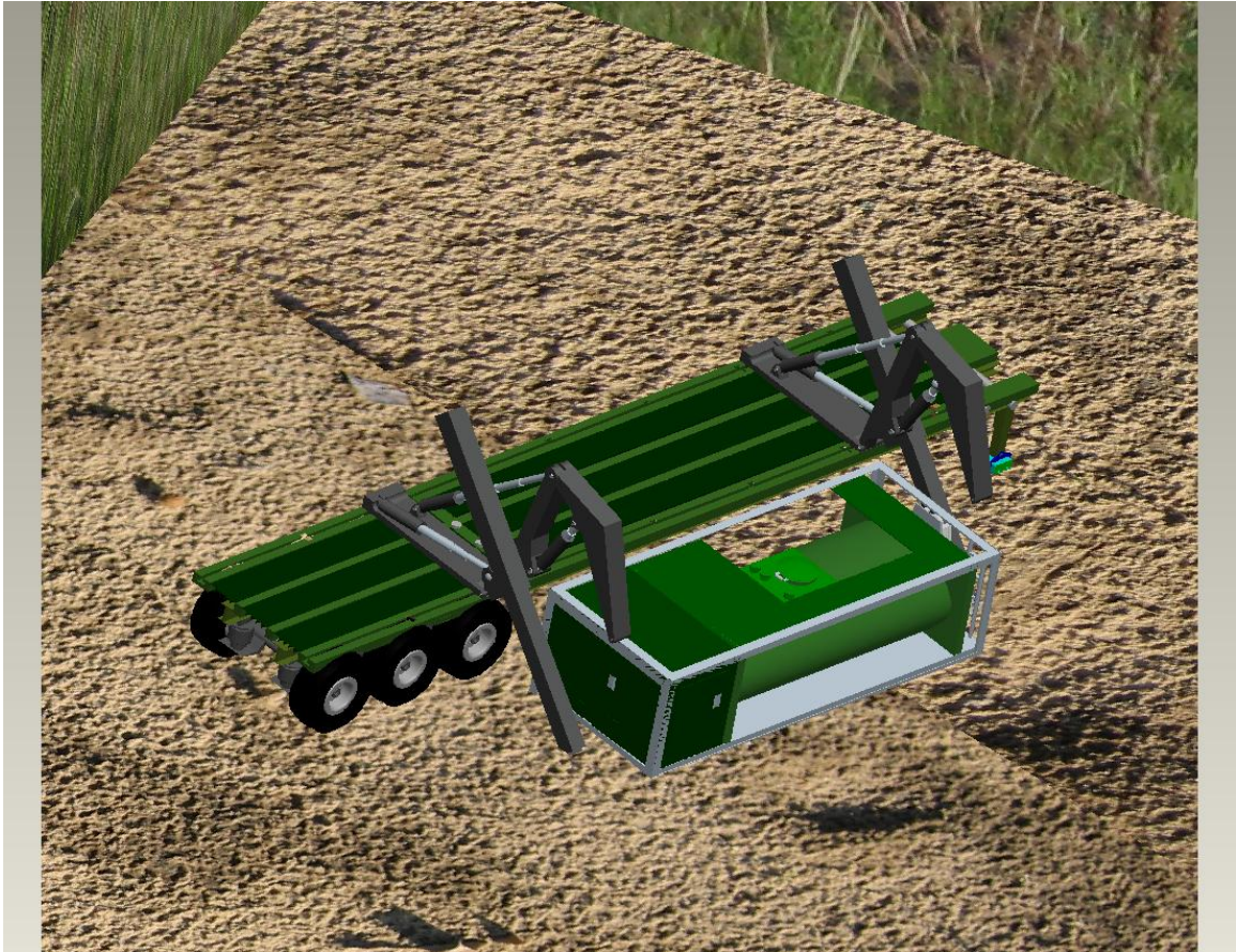
MFT Cranes in Position to Lift a Water Tank Flatrack
