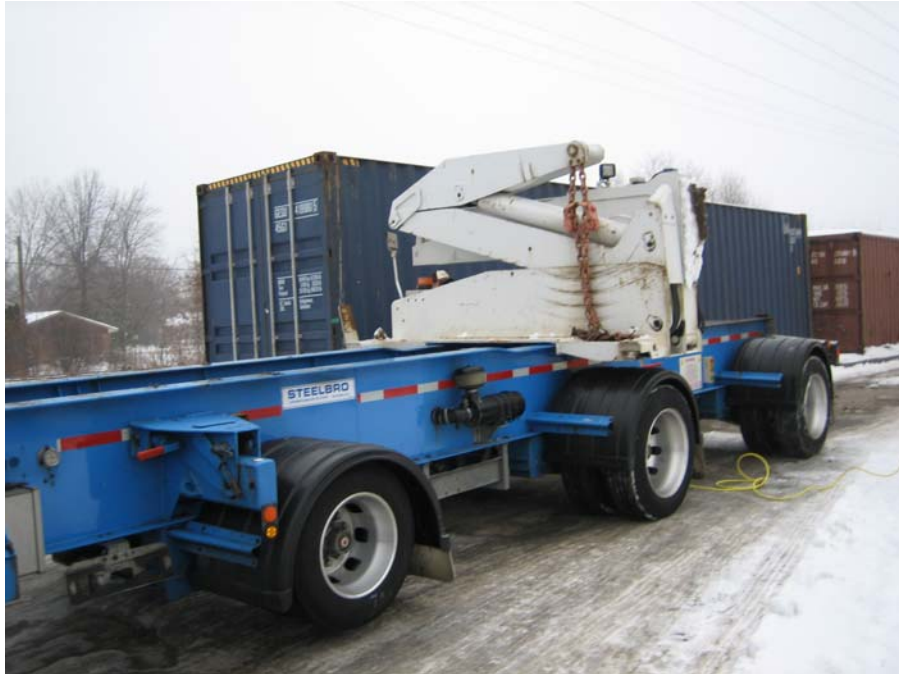
Figure 14: Rear Crane in Position to Lift 20 foot ISO
