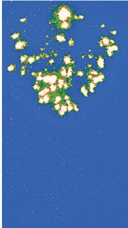
Figure 2.3: Photograph of streamer heads of a point-wire discharge in air taken with the ICCD with 0.8 ns gate. A pulse of 25 kV with a rise time of 20 ns is applied. The photo is taken 31 ns after the start of the pulse. Discharge gap is 25 mm, plane-to-plane geometry 29 .
