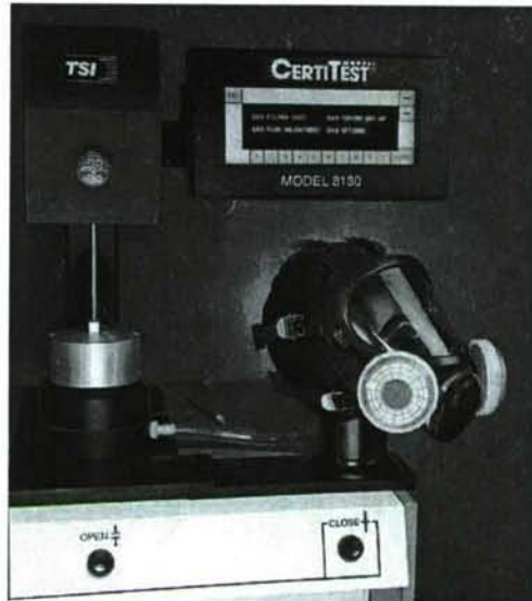
Figure 6. TSI Model 8119 Mask Leakage Tester (taken from TSI Inc., 2006)
