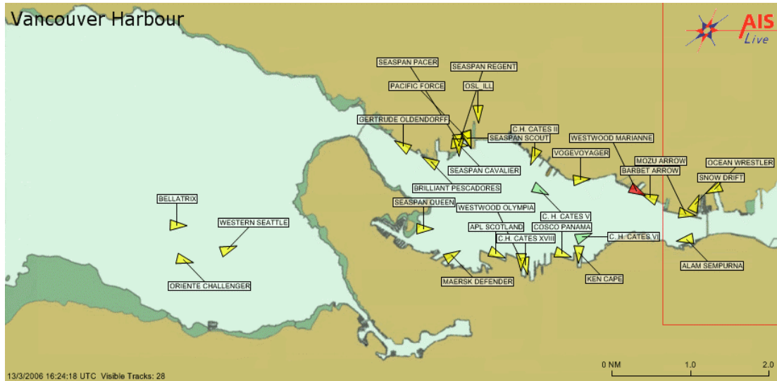
Figure 4: The positions of AIS-equipped vessels in Vancouver harbour on March 13th, 2006 are shown using isosceles triangles labelled with the vessel name [11].
