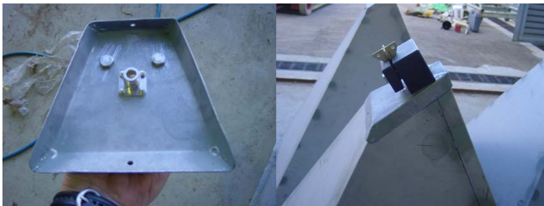
Figure 59 Details of the pyramid apex structure. On the left, the inside of the structure shows the N-connector with earthed outer connected to the sheet metal. On the right, the outside of the structure shows a nylon support block and terminal block connected to N-connector inner conductor.
