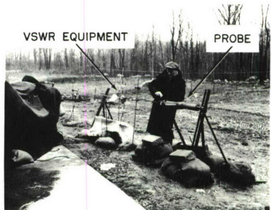
Figure 5 - VSWR and probe equipment on measurement location
