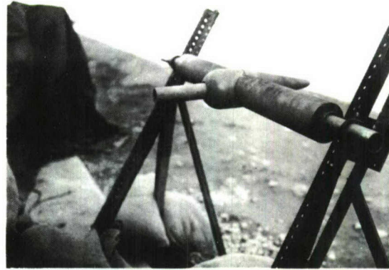
Figure 15 - X-band silicon carbide electromagnetic probe
