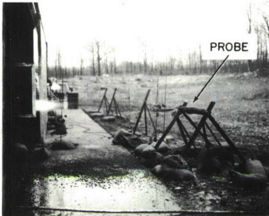
Figure 11 - K-band firing, probe outside visible portion of flame, 400-lb acid-aniline motor
