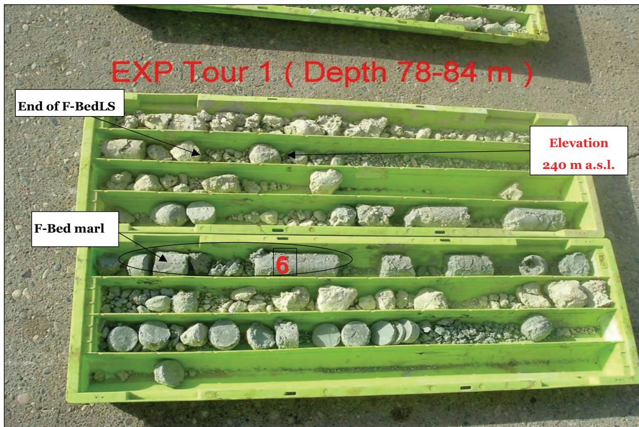
Figure 10. Core recovered from near sinkhole in residential area in 2006. Very small pieces of core and missing segments indicate RQD at or near zero, very poor rock quality.
