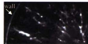
Fig. 8. OH from initial streamer distribution 500 ns after initial high-voltage pulse
