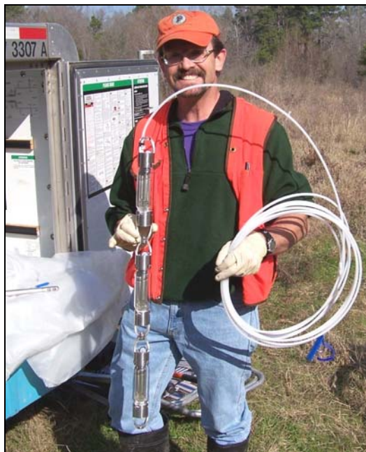
Figure 2. Assembled string of three Snap Samplers with a trigger line.
