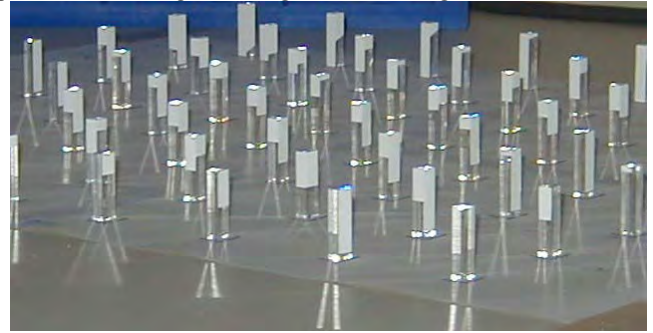
Fig.1: PQS crystal array with different white-painted reflectors or multilayer polymer mirror foil for each crystal.
