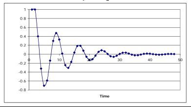
So for instance, this is the model of a classic damped pendulum. You can swing a pendulum out, think of this as over time, it will then come back and if it's in some viscous medium, it will damp out over time. And this is described by a very simple differential equation, where you can get parameters of the two dampening coefficients.
