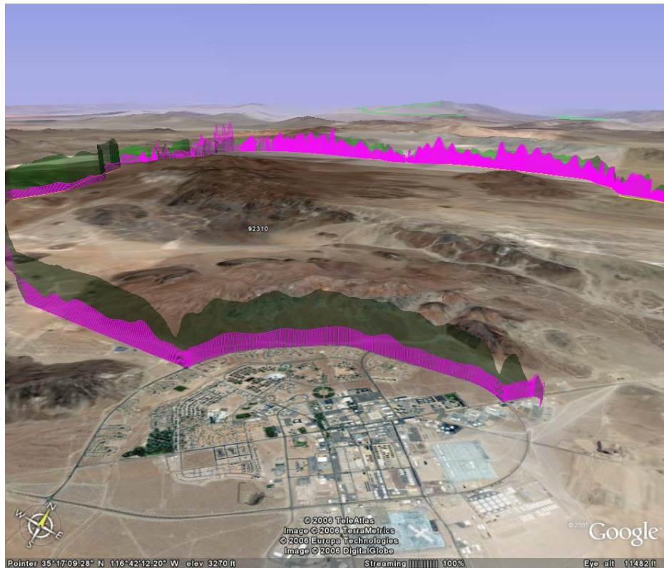
Figure 3. Latitude and Longitude Plot of Speed (green) and RMS Acceleration (pink) Values.
