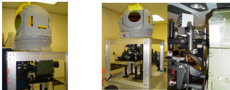
Figure 8.4 IRST with MELIOS & laser path integration
