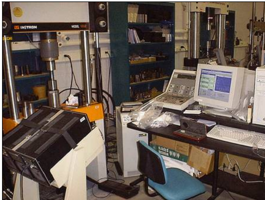
Figure 9. Typical experimental setup for fatigue testing.
