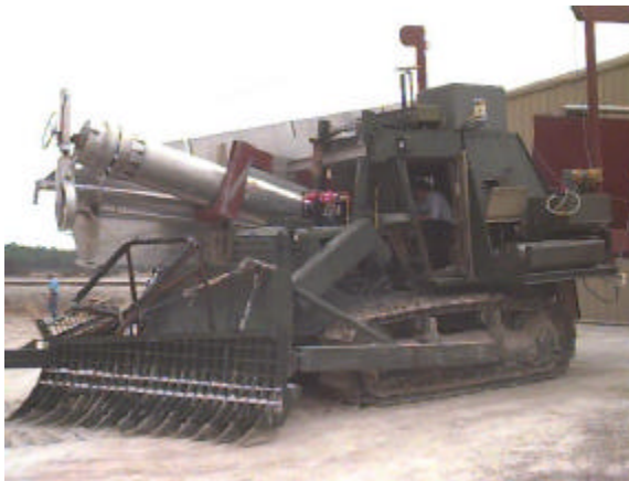
Figure 1.4: Autonomous D7G Bulldozer.
